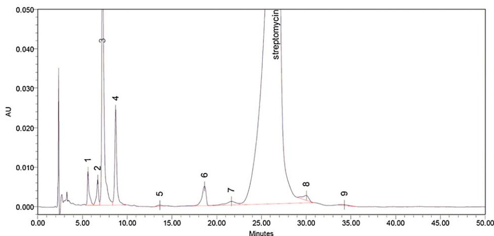
**Fig. 2.** HPLC chromatogram of streptomycin sulfate sample 10 with UV detection at 205 nm; column: Supelcosil ABZ alkylamide (250 mm × 4.6 mm, particle size 5 μm); column temperature: 45 °C; mobile phase: an aqueous solution containing 14 g/l sodium sulfate, 1.5 g/l disodium 1-octanesulfonate, 50 ml/l acetonitrile and 50 ml/l of a 0.2 molar phosphate buffer (pH 3.0).
