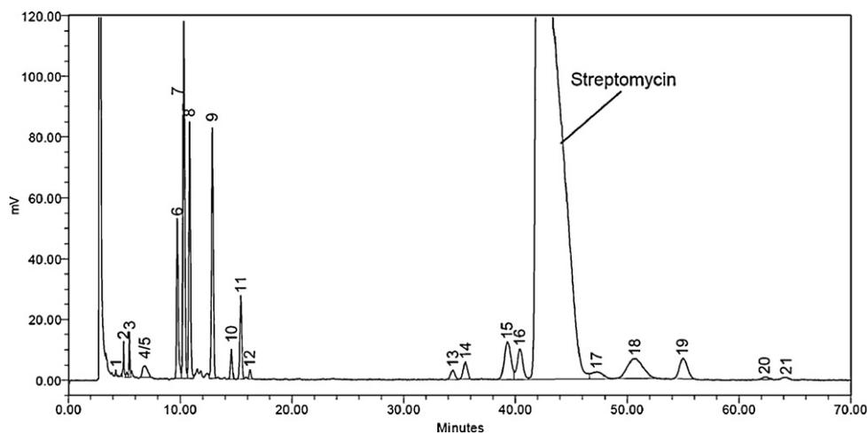
**Fig. 3.** HPLC chromatogram of streptomycin sulfate sample 4 with detection by CAD; column: YMC-Pack Pro column (250 mm × 4.6 mm; particle size 3 μm); column temperature: 40 °C; mobile phase: 20 mmol/l of PFPFA in a mixture of water/acetone 99/1 (v/v); flow rate: 0.8 ml/min; injection of 10 μl of a 5 mg/ml solution of streptomycin sulfate in water.
