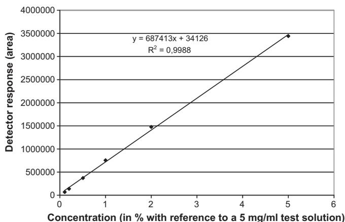
Fig. 5. HPLC-CAD calibration curve of streptomycin sulfate from 5  $\mu$ g/ml to 250  $\mu$ g/ml (6 concentration levels). Conditions as described in Fig. 3.
